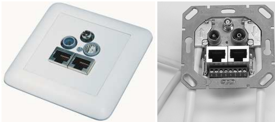
Fig. 4.5.3.1: Multimedia outlet with five sockets and terminals for twisted pair and coax cables. Photos: R&M
